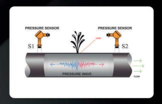
Pressure sensors installed at opposite ends of the pipeline segment will intercept and transmit the leak signal to its corresponding Asel-Tech SRU-504 remote unit. The SRU-504 is responsible for the acquisition and signal conditioning from the pressure sensors and sending the signals to a CMS. Sophisticated algorithms, Artificial Neural Networks (ANN) and other specific components of the leak detection module, process.
